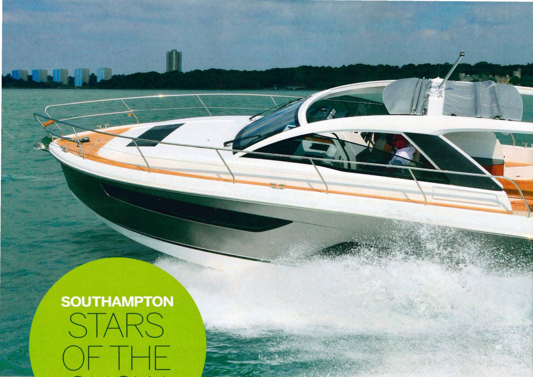
Fuller bow sections maximises the width of the forward cabin
